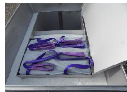
Stowage of the hoisting gear
